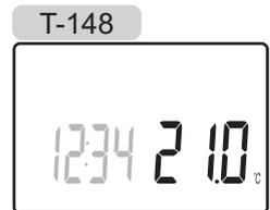
2. Press the - or + (T-149 = ▼ or ▲) button repeatedly to adjust the setpoint temperature. It will change with increments of 0.5.
