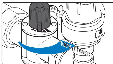
If necessary, open valve gradually for power increase
